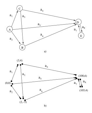
Figure 6: Simple WAN and its Constraint Graph
