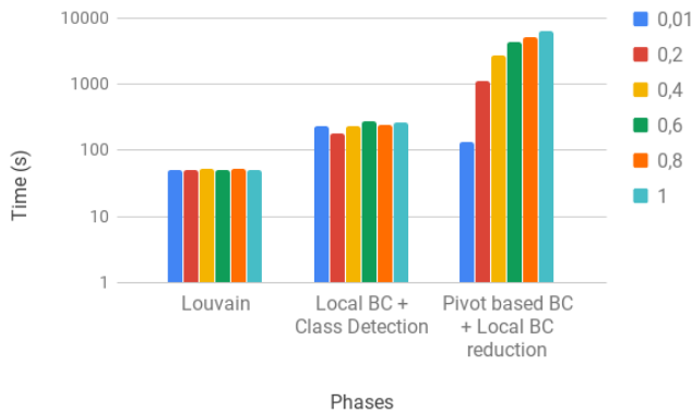
Fig. 13. Performance breakdown with 8 cores
