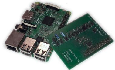
The reason for this is real-time performance. For the measures to be meaningful, we need to control the timing very precisely. This is why we don't run the usual Linux software stack, but an ad-hoc RPi firmware<sup>1</sup> instead. This program runs on two CPU cores in parallel (out of 4)
