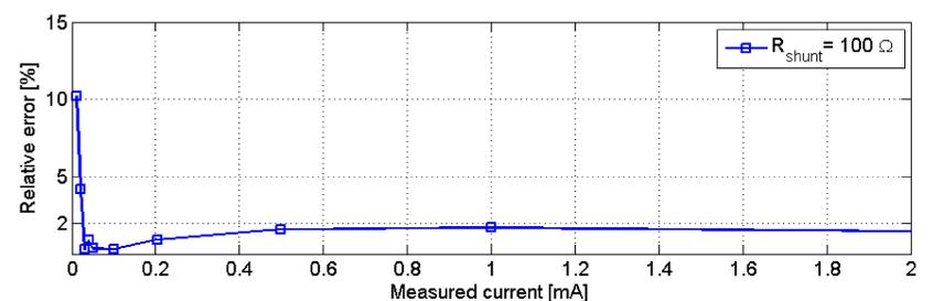
The relative error stays below 2% if the proper  $R_{shunt}$  is chosen.
