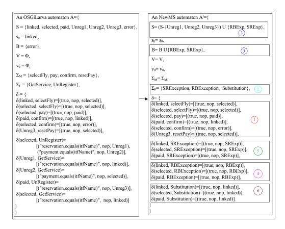
Figure 5.4: A translation example from an OSGiLarva automaton to NewMS automaton indicating algorithm steps
