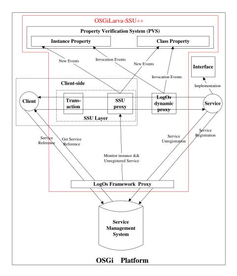
Figure 5.6: Implementation of the dynamic synthesized monitoring system
