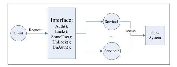
Figure 3.1: Dynamic SOA system supporting service substitution
