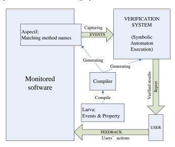
Figure 2.5: Larva system in a software system
