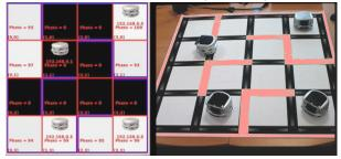
b. Snapshot at 7s, robots drop quantity 100 of pheromone (white), then evaporation decreases them (fading to black).
