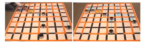
Fig. 5. a. Addition of an obstacle (tile blocked up), b. Dynamic replaning obtained from the last diffusion and updating
