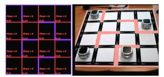
a. Snapshot of the initial state (4 robots) and the emulator interface, showing pheromone quantities (0 = black).
