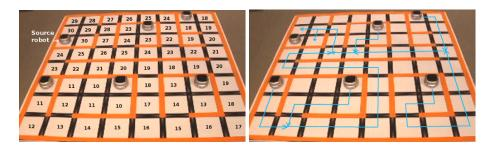
Fig. 4. a. Initial robots position, in each tile the value of  $nb_{hops}$  from the received message is written showing the first diffusion, b. *path* argument received by each robot is drawn.
