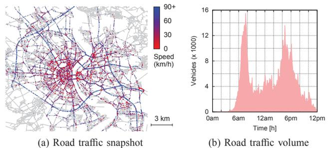
Fig. 2. Traffic characteristics for the vehicular trace from the city of Köln
