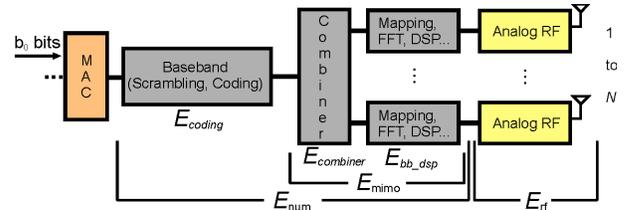
Fig. 1. A communication mode in a MIMO SDR.
